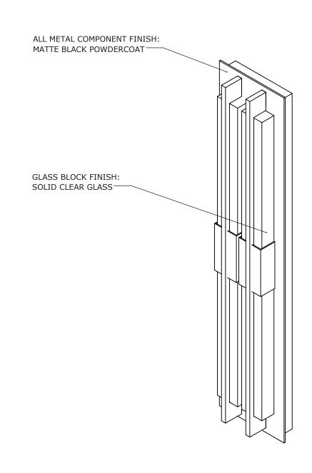
NOTES: **BLOCKING BY OTHERS DIMMING TYPE TBD INTEGRAL LED DRIVER IP65 OUTDOOR RATED**
